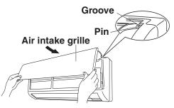
To attach the air intake grille to the indoor unit, press its bottom right and left corners as well as its bottom center into place.
